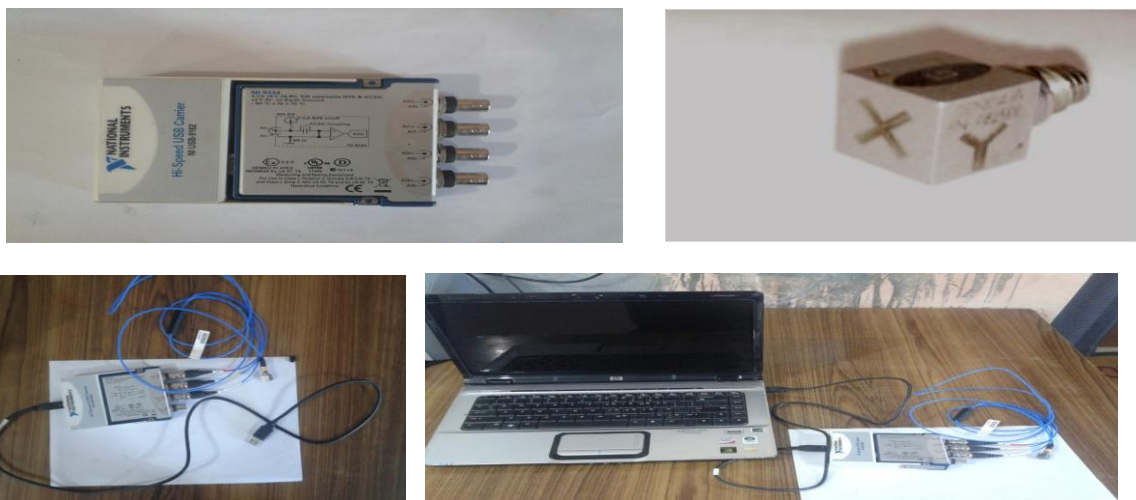
Figure 2. : The items used in data acquisition process (Triaxial transducer, Adaptor to hold transducer, data acquisition card and interfacing with Laptop)
